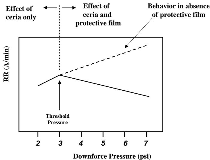
Figure 7: RR vs Pressure for a reverse-Prestonian slurry
