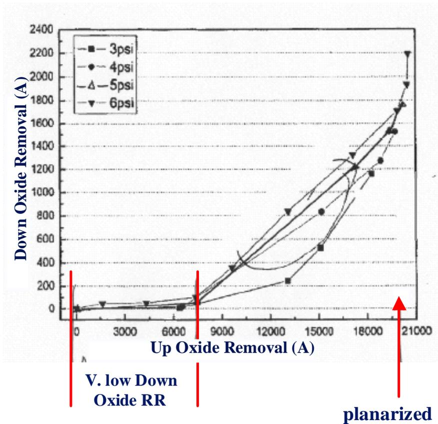
Figure 10: Down oxide vs Up oxide removal, showing High planarization efficiency (SRS-977)
