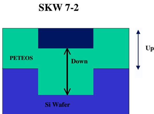
Figure 2: SKW 7-2 ILD mask cross-section (Up ~ 20,000 A)
