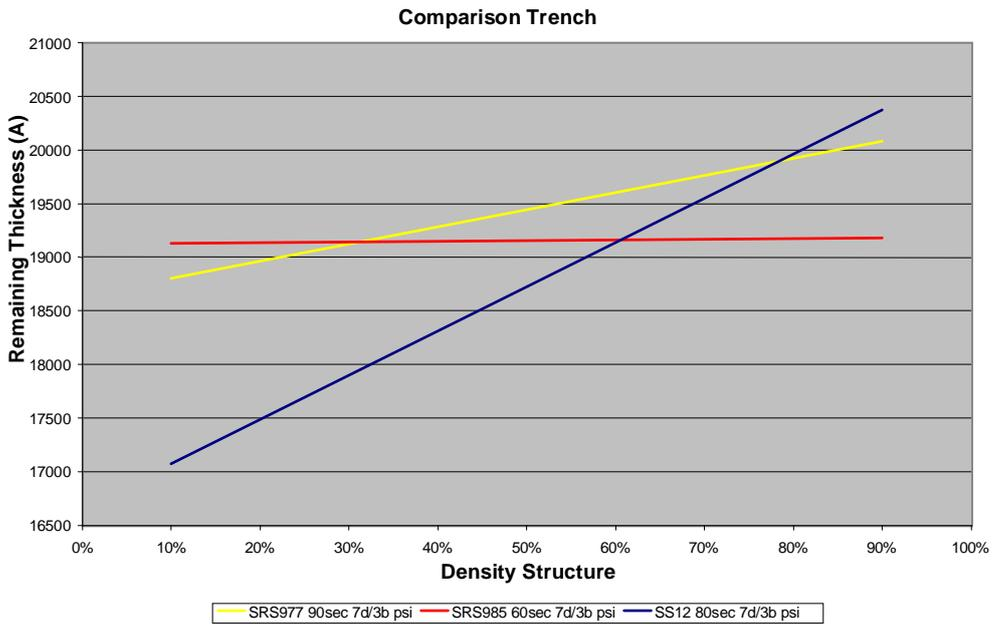
Figure 14: Pattern Dependency (SRS-985 vs SRS-977 vs SS-12)
