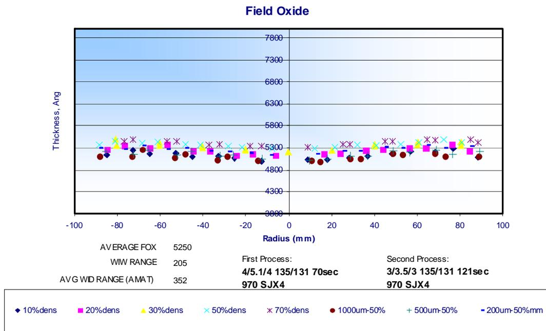
**Figure 5:** SRS-970 – 20% overpolish on Field Oxide (Fox)
