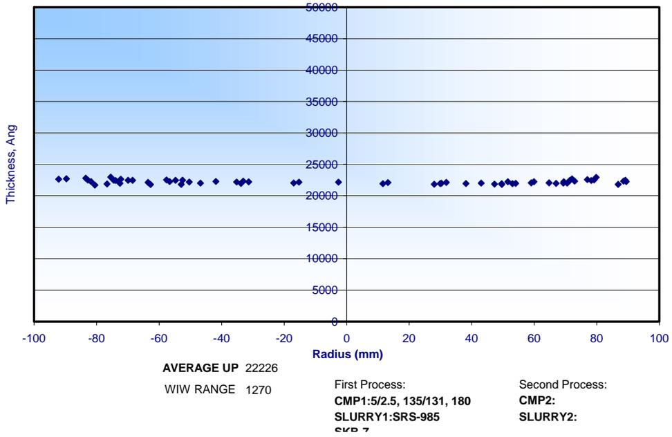
Figure 11: SRS-985 – Up oxide profile (post-polish)
