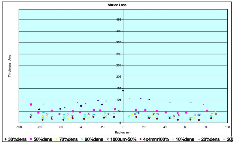
**Figure 6:** SRS-970 – Nitride loss after 20% overpolish
