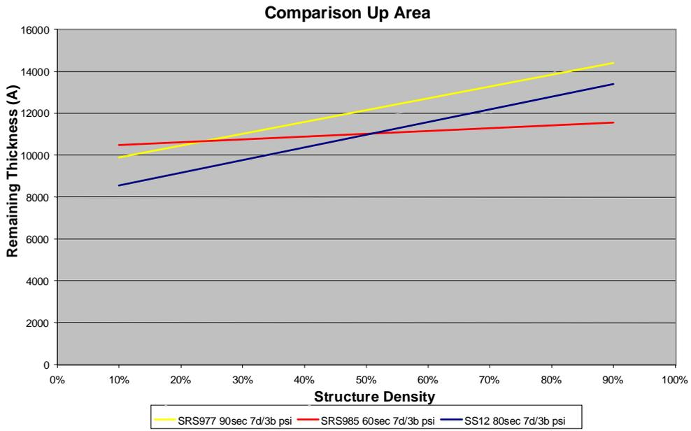
Figure 13: Pattern Dependency (SRS-985 vs SRS-977 vs SS-12)
