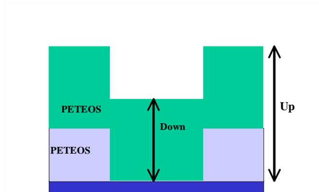
Figure 3: Customer wafer cross-section (Up ~ 43,000 Angstroms)
