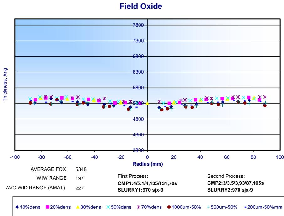
**Figure 4:** SRS-970 - polishing endpoint on Field Oxide (Fox)
