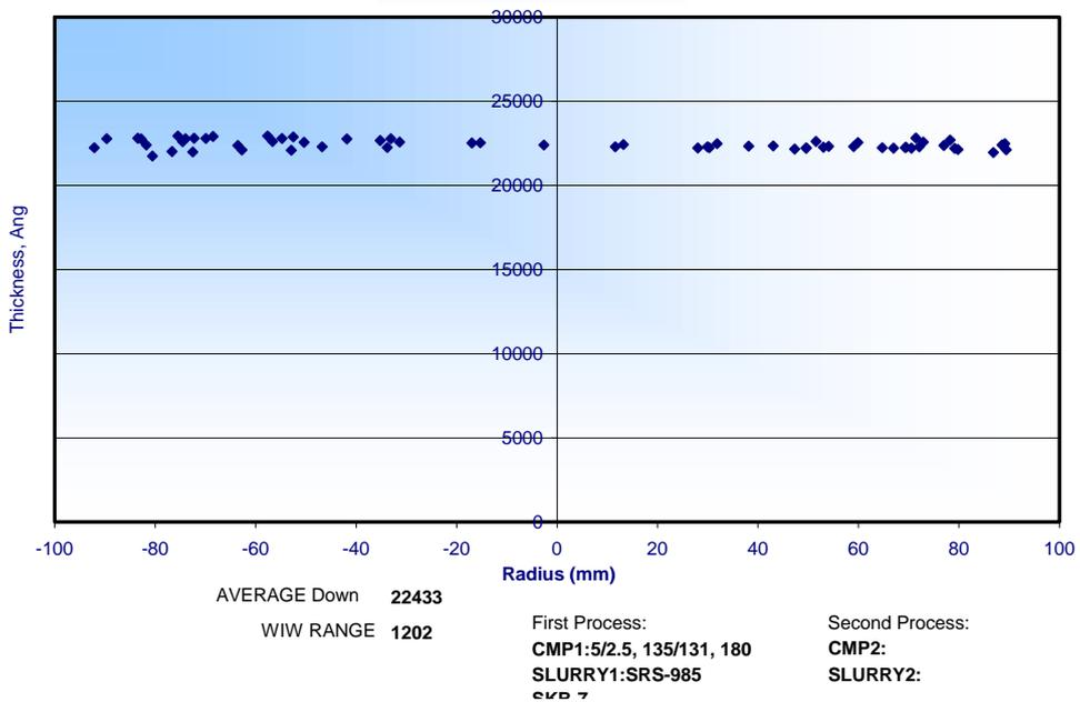
Figure 12: SRS-985 – Down oxide profile (post-polish)
